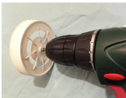
Figure 11. The FRA: Flexible Rotating Actuator.
